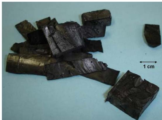
Fig. 4. Picture of a nanocomposite foamed sample (already cut into pieces prior to its characterization).
