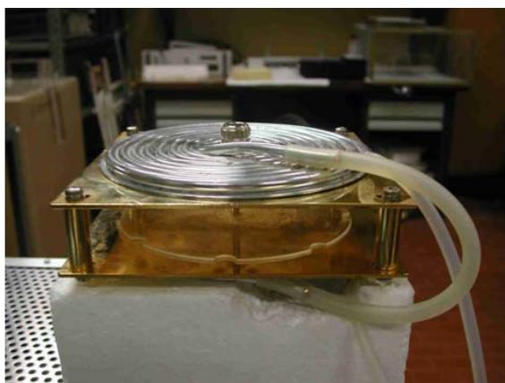
Fig. 19. Exaple of WPC with cooling system as two water spiral-plate jackets placed on external faces of WPC.
