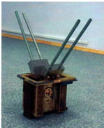
Fig. 2. Plasma dielectric antenna with four jet [8].
