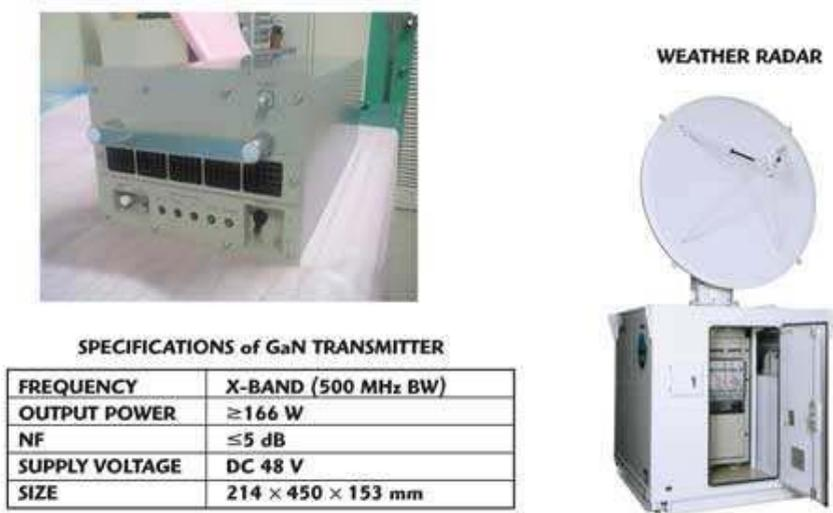
Fig. 3. Weather radar with GaN SSPA transmitter [29].
